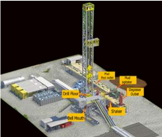
Figure 1 Location of transmitter installation
