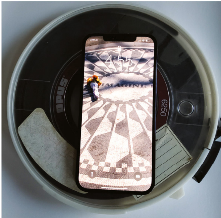
FIGURE 15.2 Nine-track magnetic tape
