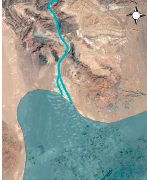
Figure 11. Large alluvial fan as an input boundary or lateral recharge, located in the northwest of Birjand aquifer. The blue line shows the groundwater lateral recharge way.
